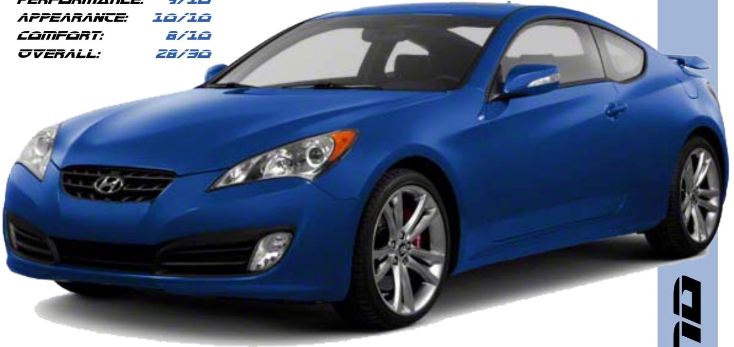
The Hyundai Genesis Coupe is available with either a 2.0-liter turbocharged four-cylinder engine or a 3.8-liter V6. The turbo ("2.0T") makes 210 horsepower and 223 pound-feet of torque, while the V6 cranks out 306 hp and 266 lb-ft of torque.
